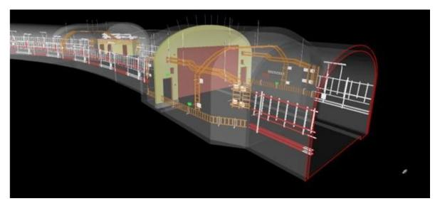
Visualization of the BIM model of the connecting tunnel for Stockholm metro (image: ©Implenia).
