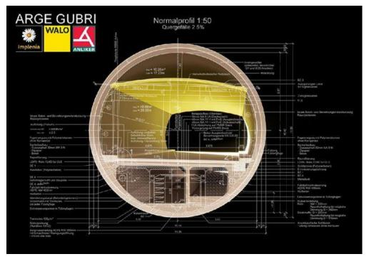
BIM visualisation of the renovation of the existing Gubrist Tunnel tubes (image: ©ARGE GUBRI).
