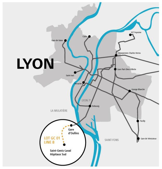
Implenia is building Lot GC 01 of the Métro Line B extension in Lyon. The lot includes a 2.4-kilometre tunnel, a new Métro station and the start shaft. Construction is scheduled to start in autumn 2018. (Image: Implenia)
